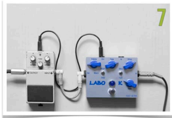
POSSIBILITY OF USING THE INTERNAL BATTERY OF THE LABO★K PEDAL TO SUPPLY A SECOND PEDAL VIA POWER-LINK CABLE
