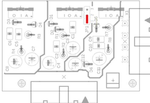
Vertical implementation of diodes
