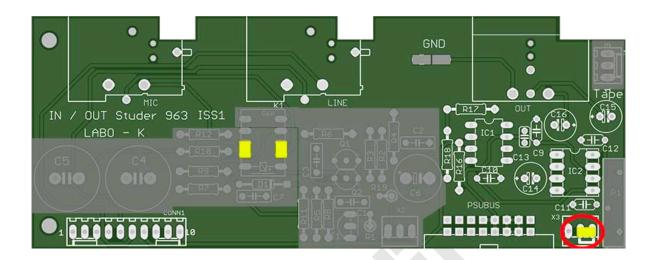
Place straps (component tails) at the points marked with yellow lines.
