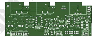
• One board for connecting : Send and Return insertion connectors. A TAPE input (Tape connector) is provided.
